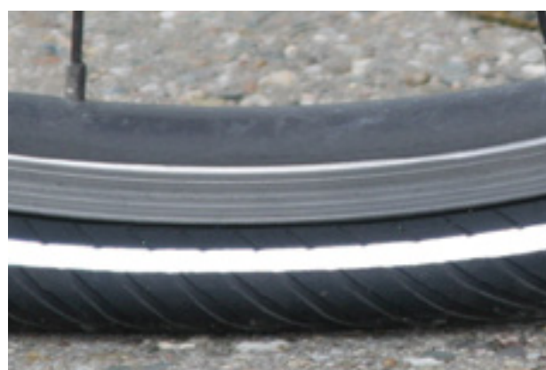
Illustration 101 : Pression largement insuffisante
