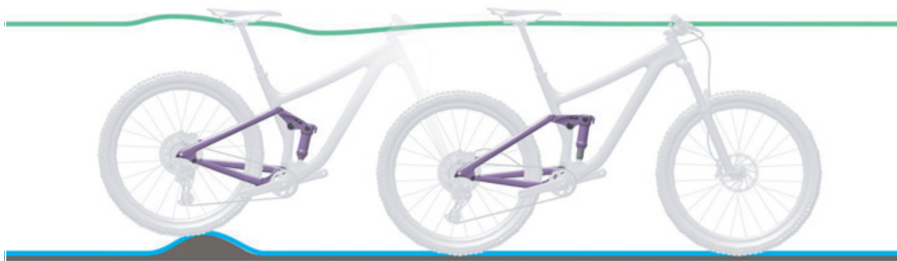
Figure 165: Optimum rear frame damper ride performance over bumps
