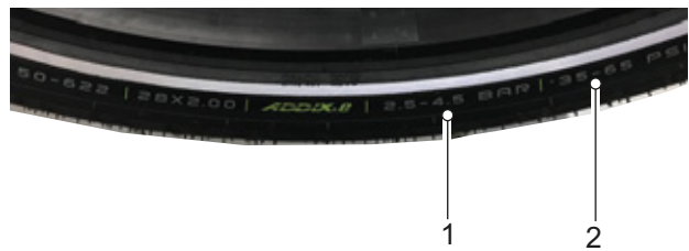
Figure 184: Tyre pressure specification in bar (1) and psi (2)
