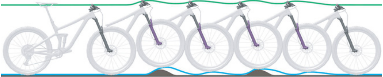
Figure 219: Suspension fork rebounding too quickly
