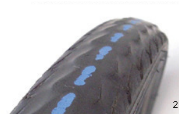
Figure 185: Tyres without a tread which can be replaced (1) and tyres with puncture protection showing through (2) must be replaced
