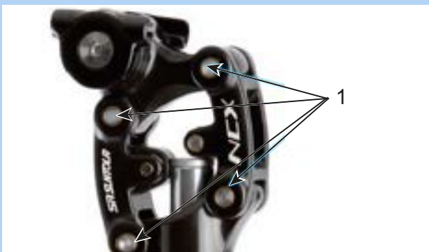
Figure 217: SR SUNTOUR suspension seat post lubrication points
