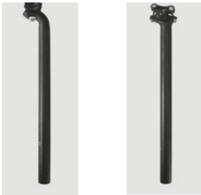
Figure 38: Example of ergotec patent seat post with either one or two seat clamp screws
