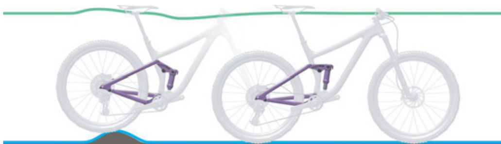
Figure 138: Optimum rear frame damper ride performance over bumps
