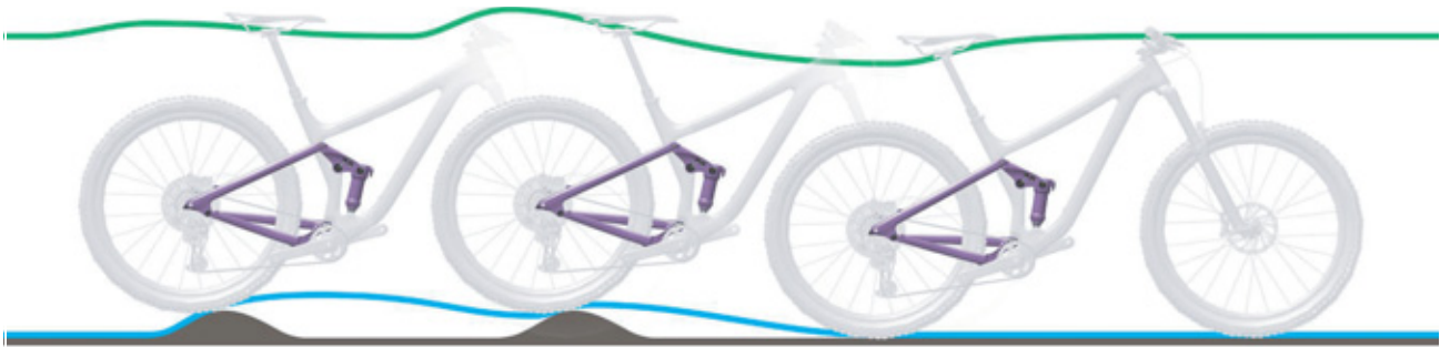
Figure 227: Rear frame damper rebounding too slowly
