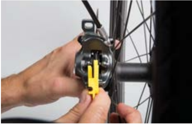
Figure 187: Checking the brake lining when fitted with the help of the transport safety wear gauge
