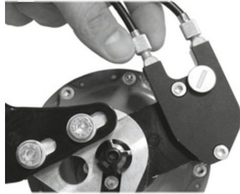
Figure 212: The tension adjuster on ROHLOFF hub versions with external switch control is located on the cable box positioned on the left-hand side
